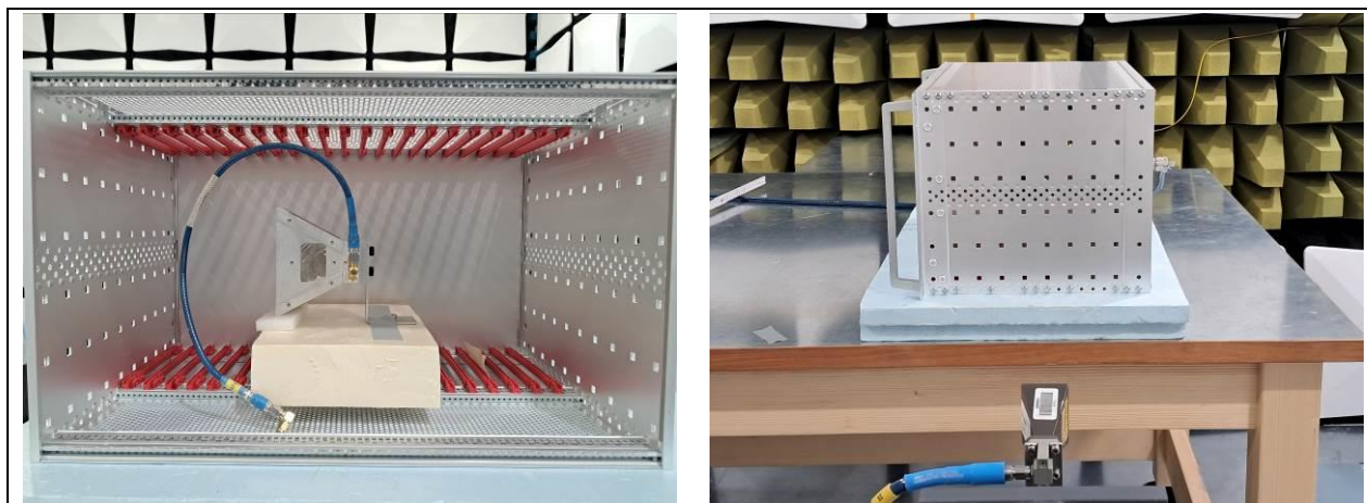
Figure 6-18: test setup horizontal, 18 – 40 GHz
