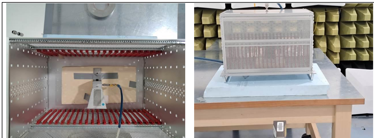
Figure 6-20: test setup horizontal, 18 – 40 GHz
