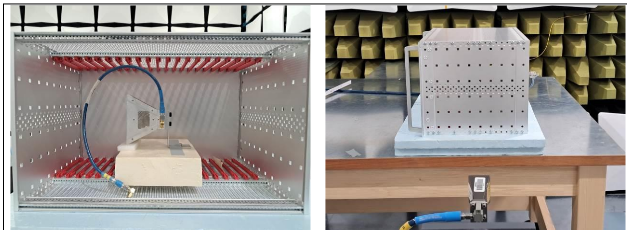
Figure 6-18: test setup horizontal, 18 – 40 GHz
