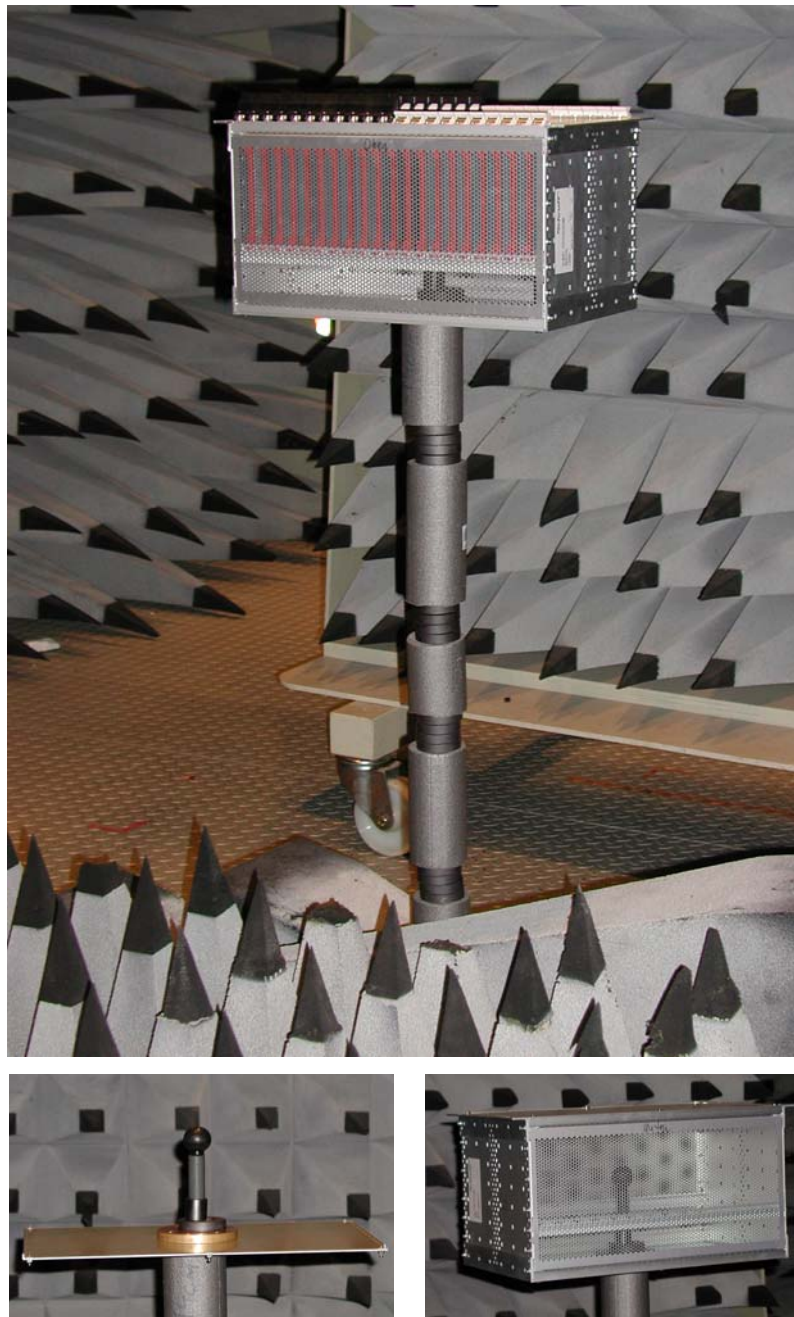
Fig. 4: EUT at the measurement position inside the anechoic chamber
