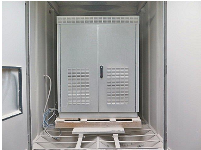
IP5X dust test
