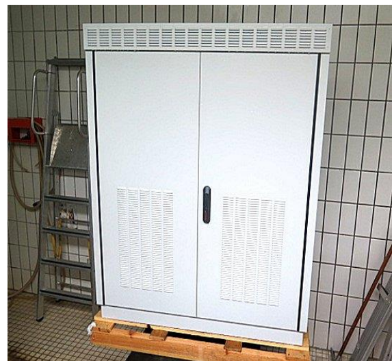
Cabinet after the IPX5 test
