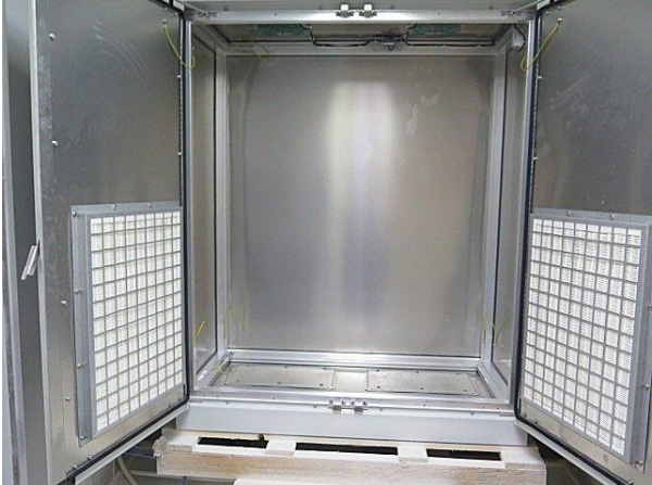
Cabinet after IP5X test
