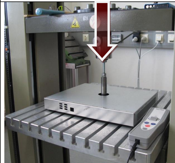
Picture 2= Force on the plate with a stamp. After all tests = no permanent deformation could be detected. Arrow = Force
