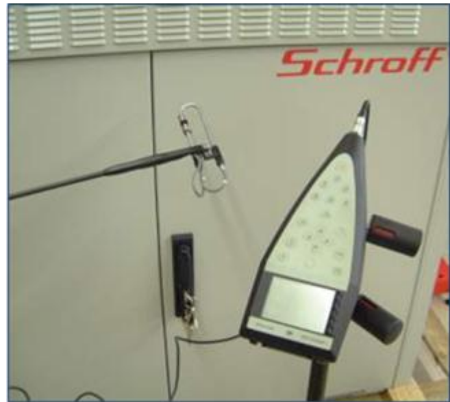
Figure 6 Test equipment acoustic noise measurements
