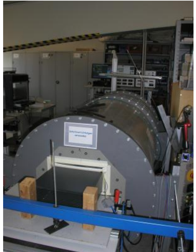
Figure 1 Interscale case fixed to Test stand for air flow volume measurement - 2
