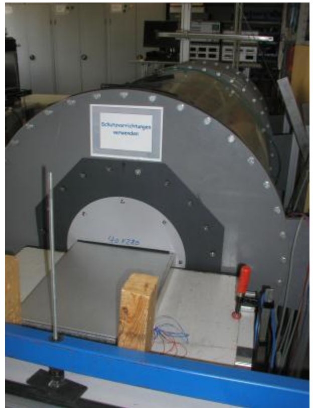
Figure 2 Interscale case fixed to Test stand for air flow volume measurement - 2
