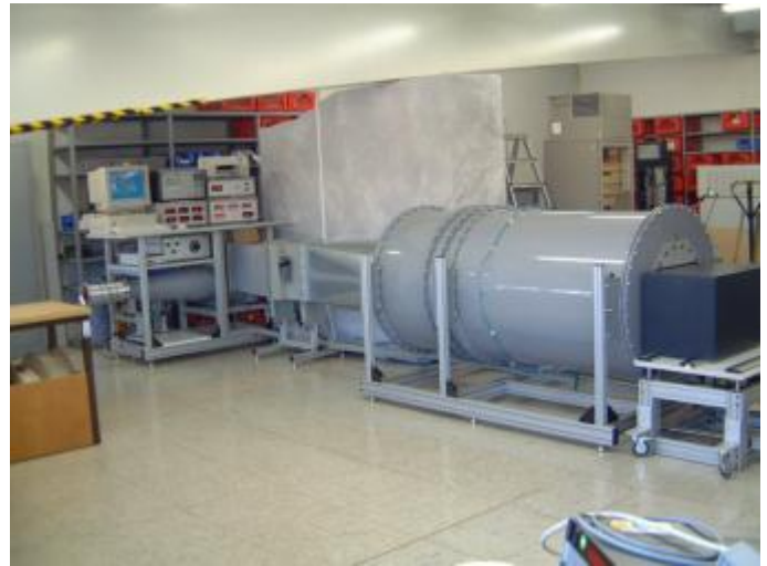
Figure 3 Test stand for air volume measurements
