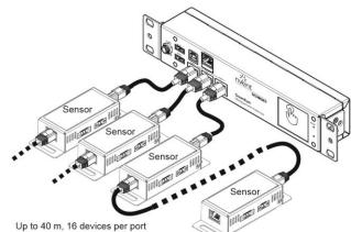
With 1:1 CAT 6 patch cables, up to 16 sensors can be linked together and connected to SCHROFF environmental monitoring devices
